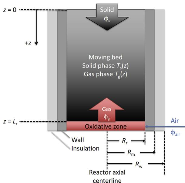
Fig. 2. A schematic representation of the modeling coordinates in the reactor.
