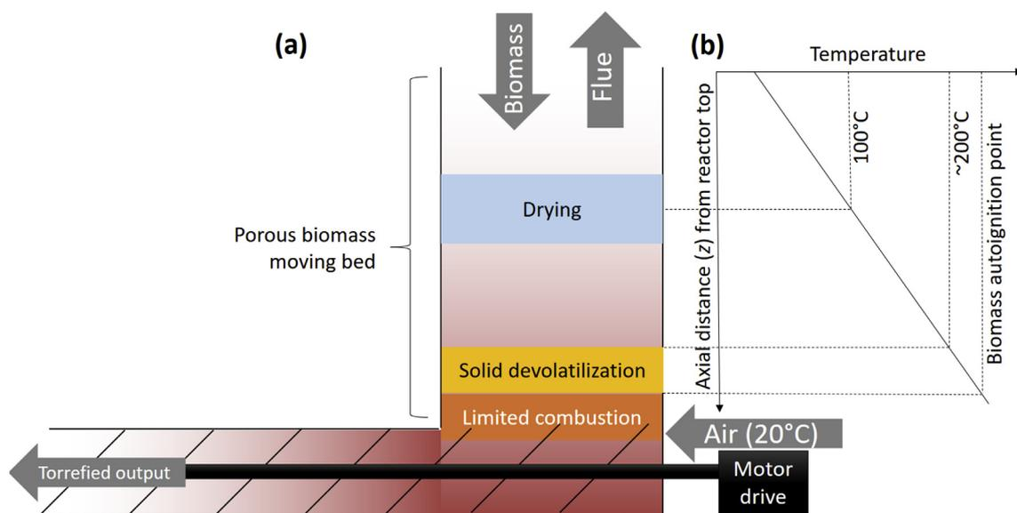
Fig. 1. A reproduction of the same figure from Part I of this study, showing (a) a schematic of an oxygen-lean moving bed torrefaction reactor design, and (b) guesSED axial temperature profile and behaviors within the reactor.
