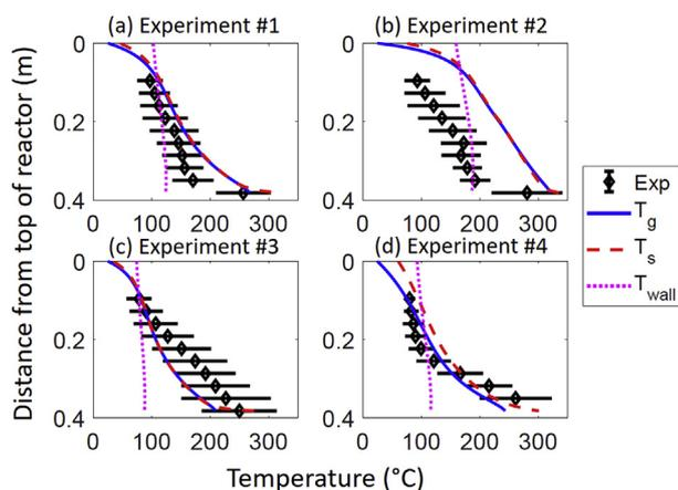
**Fig. 3.** Axial steady-state temperature profiles for simulated gas phase (blue solid line), simulated solid phase (red dashed line), and simulated wall temperature (purple dotted line) in the biomass torrefaction reactor as compared to that measured on a profile thermocouple (black open diamonds with error bars) in our experimental set-up. (For interpretation of the references to colour in this figure legend, the reader is referred to the Web version of this article.)
